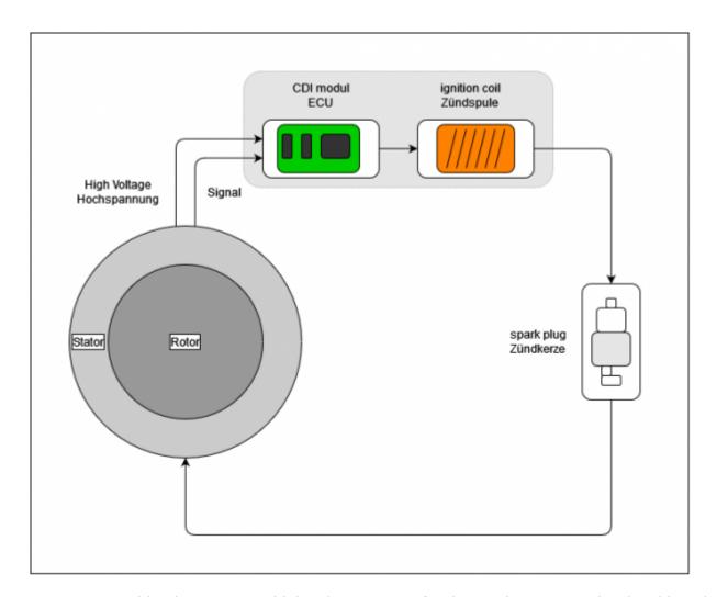
The stator-rotor-combination creates a high voltage source for the spark energy and a signal impulse for triggering the ignition point. The CDI modul (also called ECU = electronic control unit) stores the spark energy, until the triggering signal releases the current to the ignition coil. In this coil the voltage gets transformed to several 10k volt and then creates the spark in the spark plug. This is the moment where the combustion in the engines is started.
